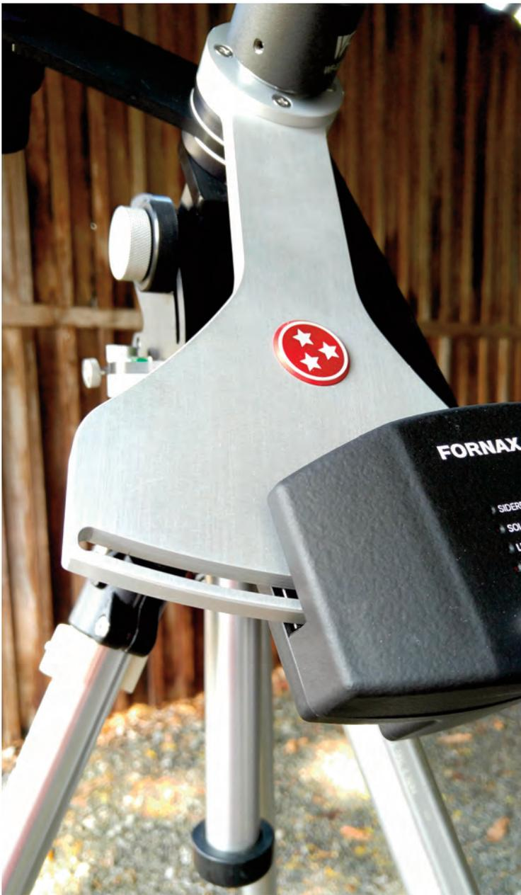
**Image 3 -** The drive-disc bearing surface of the Lightrack II's virtual disc section is actually the inner surface of the slot formed along the outer (bottom) edge, which position serves to protect the critical drive-bearing surface. The drive roller is positioned inside of the black motor housing.
