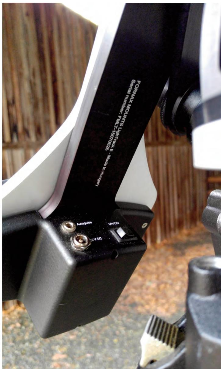
**Image 7 - The mount's on/off button, 12-volt DC power port and custom autoguider port are located within easy reach on its underside.**
